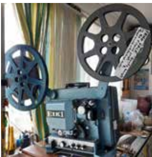
Above: An Eiki self-threading 16mm projector, with a just-screened film reel aboard. Ideally, you should darken the room before screening your films.
